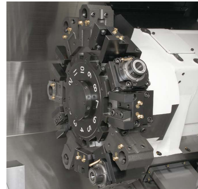
V12 radial multitasking turret
