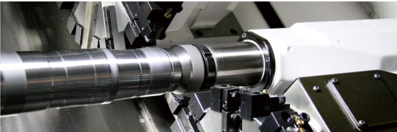
Example of high accuracy machining (LU3000 EX actual data)
