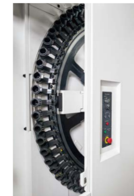
Disk system ATC magazine (64 tools: option)
