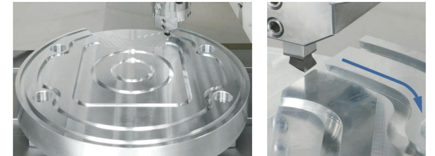
The cutting edge direction is controlled to match the groove
