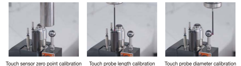
Touch sensor zero point calibration Touch probe length calibration Touch probe diameter calibration
