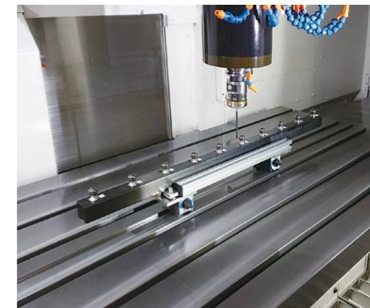
Linear axis error measurement using the accuracy master (ball beam) and touch probe
