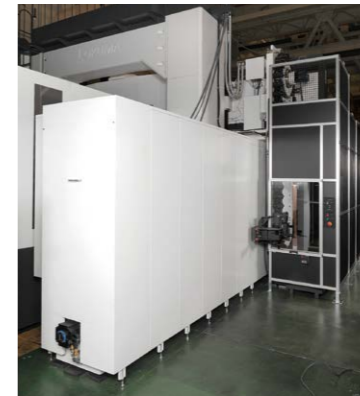
The attachment head station is set at the rear of the ATC magazine behind the column.
