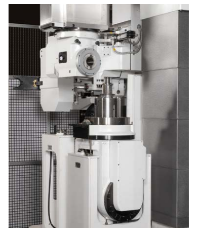
Changing heads: B-/C-axis universal index to 90° angular
