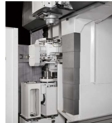
Auto attachment head change: Attachment station moves near the spindlehead below the crossrail, then attachments are changed.
