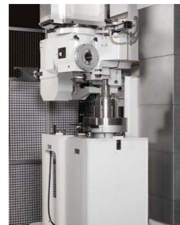
Changing heads: extension to 90° angular
