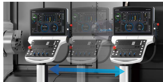
The panel can be moved left or right, providing excellent access to the spindle Note: The operation panel of the MULTUS U3000 (distance between centers: 1000 mm) cannot be moved left or right.
