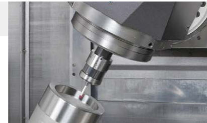
Inner diameter measurement of angled holes
