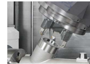
Turning can be done on a sloped axis
