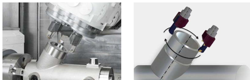
Turning can be done from a inclined axis
