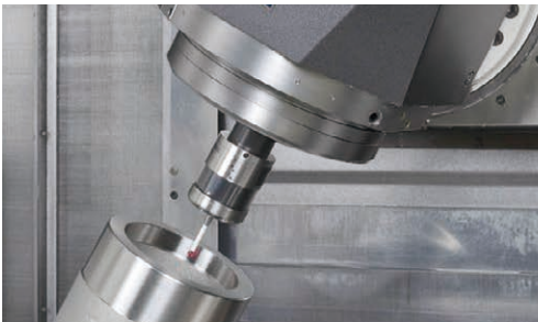
Inner diameter measurement of angled holes The image shows a similar model, the MULTUS U3000
