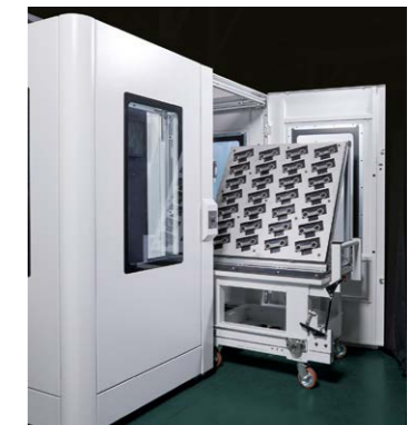
A dedicated fixture attached to the tilted cart.
