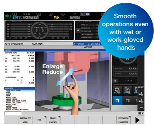
Note: 19-in. operation panel (option) screen shots. Collision Avoidance System (option) shown above.
