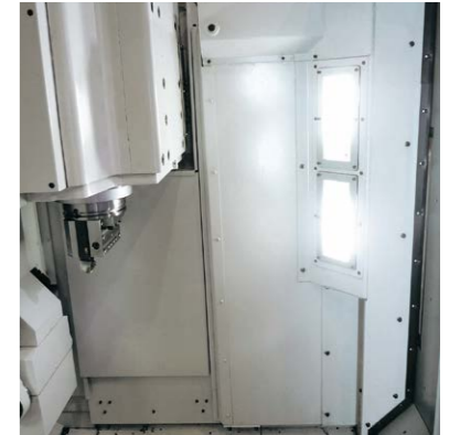
ATC-cover-side angled double-LED lamp—easier tool edge checks, etc
