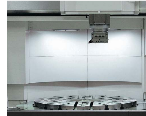
2 LED lamps under crossrail
